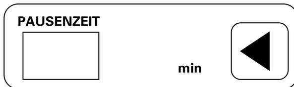
There is no separate function field for this function. The aeration time is set in the function field for pause time.
